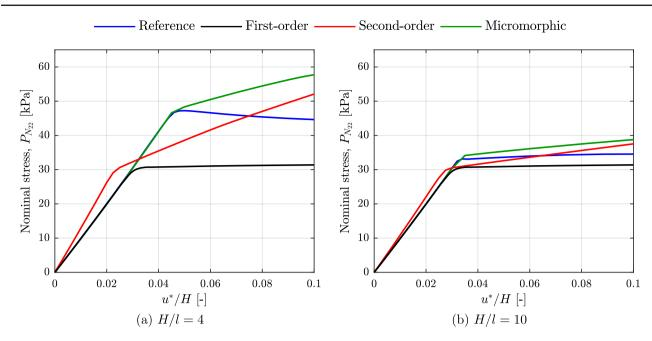
Fig. 16 Finite specimen compression case. Stress-strain diagrams corresponding to scale ratios **a** 4, and **b** 10, obtained by the first-order, second-order, and micromorphic homogenization schemes, as compared to the reference ensemble averaged solution
