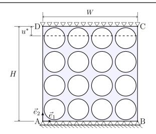
**Fig. 14** Finite specimen compression case. Illustration of the simulation  $4l \times 4l$  domain subjected to a vertical compressive load. The two lateral edges, AD and BC, are free surfaces
