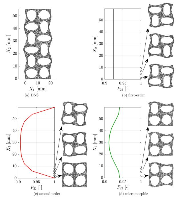
**Fig. 6** Uniform compression case. Deformed configuration of an infinitely wide specimen with scale ratio H/l = 6, subjected to 7.5% nominal compressive strain. **a** DNS solution corresponding to zero microstructural translation  $\vec{\zeta} = \vec{0}$ .  $F_{22}$  component of the macroscopic
