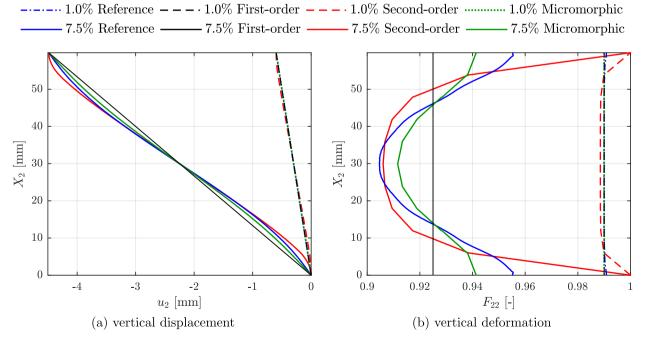
Fig. 5 Uniform compression case. Comparison of **a** vertical displacement component  $u_2(X_2)$ , and **b** deformation gradient  $F_{22}(X_2)$  over the specimen's height. Overall applied compressive strain corresponds to 1 and 7.5%, for a specimen with scale ratio H/l = 6
