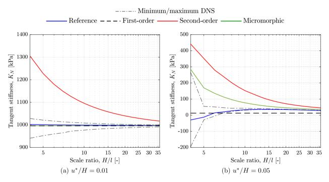
Fig. 18 Finite specimen compression case. Tangent stiffness in the **a** pre-bifurcation and **b** post-bifurcation regime as a function of the scale ratio  $H/l \in [4, 36]$
