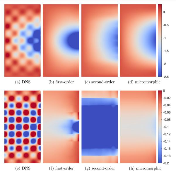
Fig. 19 Finite specimen compression case. Resulting field plots for  $u^*/H = 0.075$  and H/l = 10, for the right half of the domain. The top row corresponds to the horizontal displacement component  $\vec{u} \cdot \vec{e}_1$  [mm] for a DNS, b first-order, c second-order, and d micromorphic simulation. The bottom row corresponds to the  $F_{22} - 1$  [–] component
