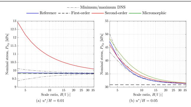
Fig. 17 Finite specimen compression case. Nominal compressive stress in the **a** pre-bifurcation and **b** post-bifurcation regime as a function of the scale ratio  $H/l \in [4, 36]$
