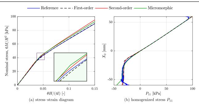
Fig. 12 Uniform bending case corresponding to scale ratio 12. a Stress-strain diagram; a close-up of the bifurcation point in the inset. b  $P_{11}$  stress component along the vertical reference coordinate  $X_2$  at  $\theta H/(4l) = 0.1125$
