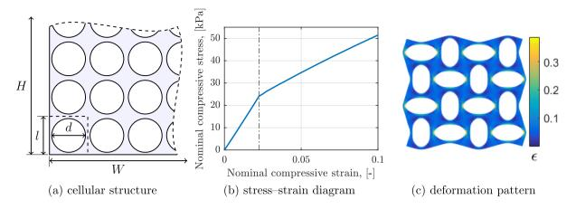
Fig. 1 a Sketch of the two-dimensional elastomeric metamaterial, including the geometrical parameters, and b corresponding stress-strain response in compression. c Deformation pattern of a  $4 \times 4$
