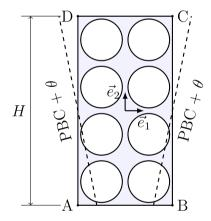
**Fig. 10** Uniform bending case. A sketch of the simulation domain and boundary conditions for a specimen with scale ratio H/l = 4. Superposed periodic boundary conditions are enforced along the vertical edges AD and BC to mimic an infinitely wide structure
