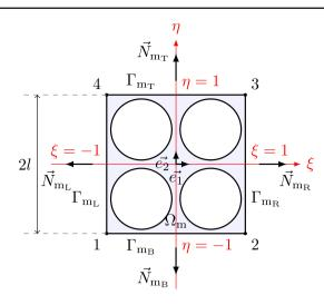
Fig. 3 Schematic representation of the adopted square RVE with domain  $\Omega_m$ , consisting of  $2 \times 2$  unit cells. The RVE has four corner points, 1, ..., 4, four boundary segments  $\Gamma_{m_{\bullet}}$  with associated outer normals  $\vec{N}_{m_{\bullet}}$ , where  $\bullet$  represents right (R), left (L), top (T), and bottom (B) edges, and is parametrized by two normalized coordinates  $\xi \in [-1, 1]$  and  $\eta \in [-1, 1]$
