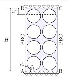
**Fig. 4** Uniform compression case. A sketch of the considered simulation domain and boundary conditions for a specimen with scale ratio H/l = 4. Periodic boundary conditions are enforced along the two vertical edges AD and BC, representing an infinitely wide structure
