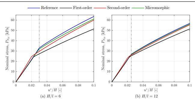
Fig. 7 Uniform compression case. Stress-strain diagram for scale ratios **a** H/l = 6 and **b** H/l = 12, obtained via DNS and the first-order, second-order, and micromorphic homogenization schemes
