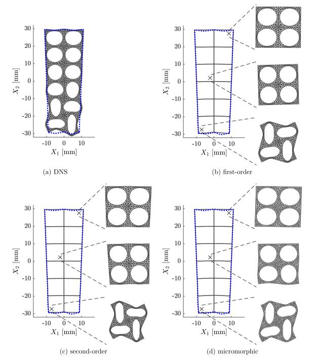
**Fig. 11** Uniform bending case. An infinitely wide specimen with scale ratio 6 bent up to  $\theta H/(4l) = 0.1125$ . **a** DNS solution with zero microstructural shift  $\vec{\xi} = \vec{0}$ . The macroscopic deformed structures including deformed RVEs corresponding to three macroscopic inte-
