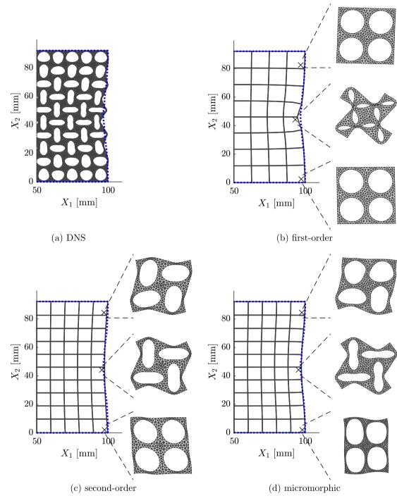
**Fig. 15** Finite specimen compression case. Right half of a deformed  $10l \times 10l$  specimen obtained by a DNS subjected to  $u^*/H = 0.075$  compressive strain, corresponding to a zero microstructural translation  $\vec{\xi} = \vec{0}$ . The right half of the macroscopic deformed structure, including deformed RVEs positioned at three macroscopic integration
